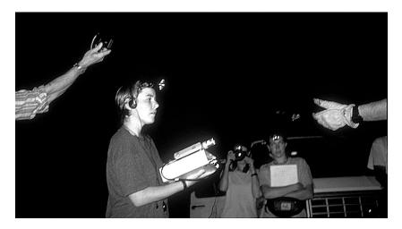
Figure 16: Using a bat detector in the field to record echolocation calls of a bat as it is released.
