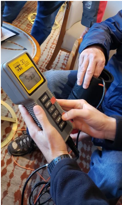
Checking Water Temperature
