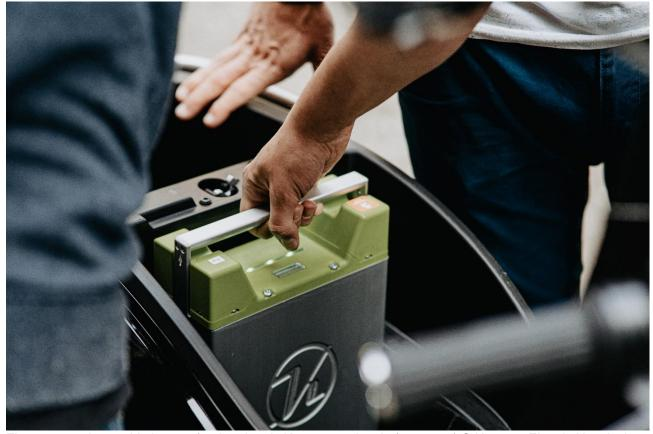
Figure 2 a rechargeable battery for the electric Kumpan 54 Iconic (a scooter) © Kumpan Electric Unsplash
