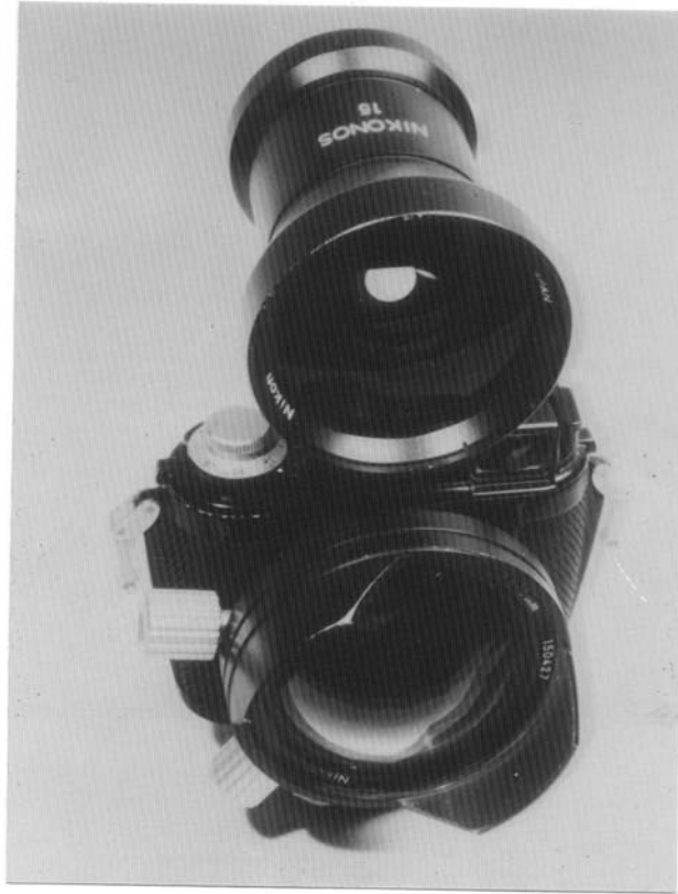
Figure 10 A Nikonos II with a 15mm Nikonos lens and a Nikonos optical viewfinder.
