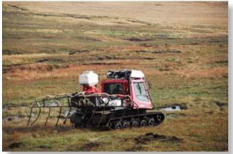
Applying heather seed into colonisation gaps on wildfire site using low ground pressure vehicle
