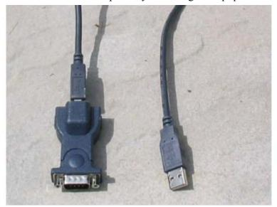
Figure 11-2 Serial - RS232 9 pin male to USB converter. The RS23 serial connector is shown on the left and the USB connector is shown on the right. The RS232 connector receives the female GPS connector and transfers the data through the USB port of the PC.
