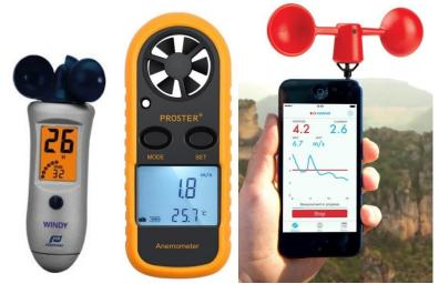
With anemometers, you generally get what you pay for. Cup anemometers (left) are best, because they work whatever direction the wind is coming from. However, they can be expensive and are very delicate. Propeller anemometers (centre) can be much cheaper. However, the propeller has to be pointed into the wind to get a good reading; the wind direction can be hard to judge when the wind is weak or gusty.
