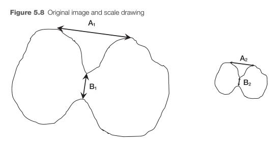
Another way of representing the scale factor would be to say that the scale of the drawing is 1:3. Note that, in this ratio, the first number represents the dimension of the scale drawing and the second number represents the dimension of the original. Other examples of scales as ratios would be a model aeroplane with a scale of 1:72 and a map with a scale of 1:50000.
