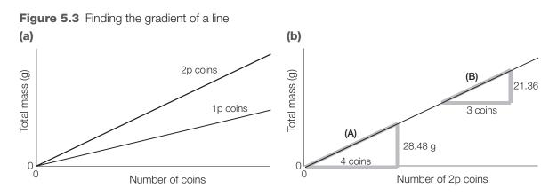
Figure 5.3b shows how the gradient of this line can be measured: it is the increase in the variable on the *vertical axis* or *y-axis* divided by the corresponding increase in the variable on the *horizontal axis* or *x-axis*.
