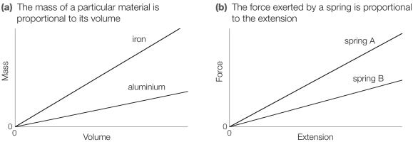
An example of a relationship derived from experiment is Hooke's Law. By experiment, it was found that the force exerted by a spring is proportional to the extension (within the elastic limit of the spring). The constant of proportionality is called the spring constant and it is a characteristic of a particular spring: the larger the spring constant, the stiffer the spring (Figure 5.5b).
