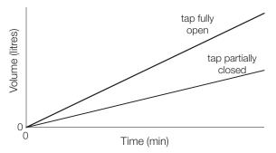
Since this is a change over time, the gradient represents a *rate* of change. In this case, the gradient is the *flow rate* of the water and is measured in litres/min. Both lines are straight and
