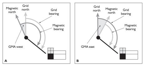
Figure 6.4 Grid magnetic angle (GMA): (a) magnetic bearing = grid bearing + GMA; (b) magnetic bearing = grid bearing - GMA
