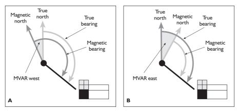
Figure 6.5 Magnetic variation (MVAR): (a) magnetic bearing = true bearing + MVAR; (b) magnetic bearing = grid bearing - MVAR
