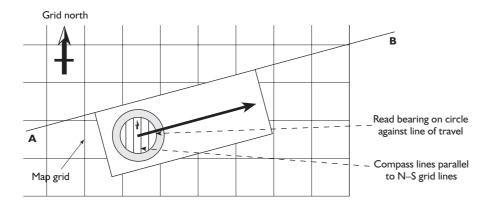
Figure 6.2 Grid bearings
