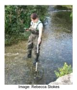
Flow meter: Used to measure the velocity of moving water.
