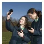
**Light meter:** Used to measure the amount of light or cloud cover.
