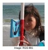
**Clinometer:** Used to measure the angle of a slope.
