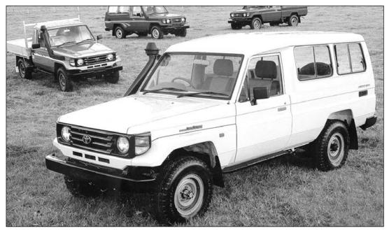
Figure 28.9 Classic robust simplicity – the Australian spec Toyota Type 78 even comes with long-range fuel tanks as standard. This one has coil springs at the front. Never imported into UK, earlier all-leaf-sprung Type 75 in diesel form is highly valued in continental Europe for expedition work (© Tom Sheppard)
