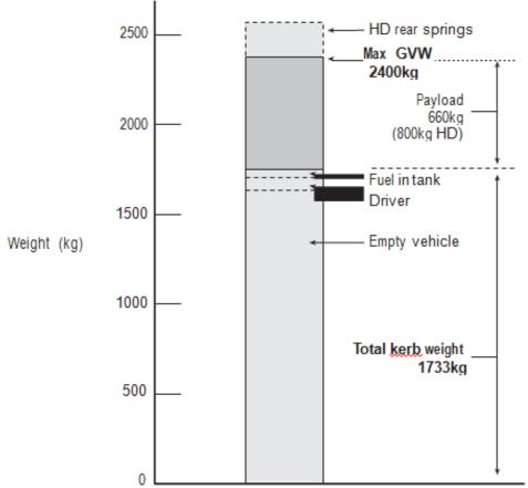
Figure 28.1 How a vehicle's GVW (gross vehicle weight) is made up. Never exceed it by adding too much payload. Figures shown are for Defender 90
