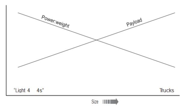
Figure 28.6 The size trade-offs: power:weight ratio and payload
