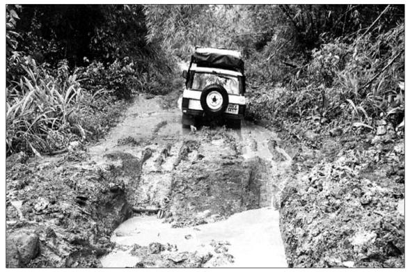
Figure 28.8 A 4 x 4 is best. Here, as with rock crawling or steep washouts, low-range gears are virtually essential ( $^{\circ}$  Tom Sheppard)
