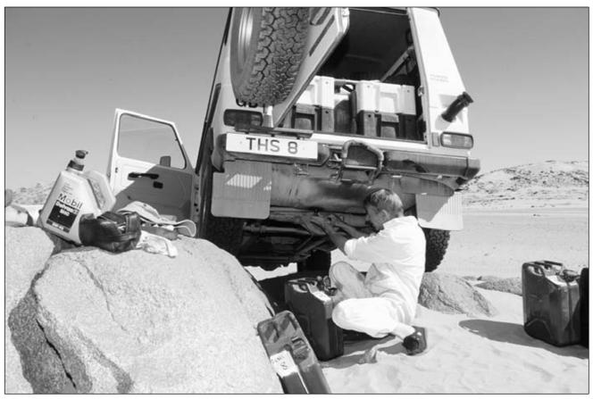
Figure 28.11 Be ready to improvise. Electronic control unit (ECU) defaulting to "limp home" and suspected fuel contamination demanded drain and filter for all fuel on board – an all-day job. Rocks provide handy ramp for jerry can access; failing that a dig-down hole would have sufficed (© Tom Sheppard)
