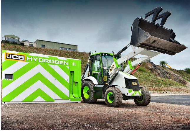
Figure 2 a JCB hydrogen-powered backhoe loader © JCB
