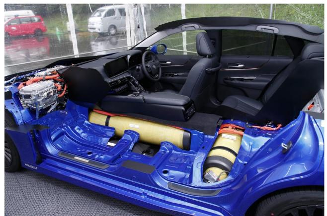
Figure 1 the Toyota Mirai. The yellow tanks are for storing hydrogen. The fuel cells are located in the engine bay © Toyota 2021
