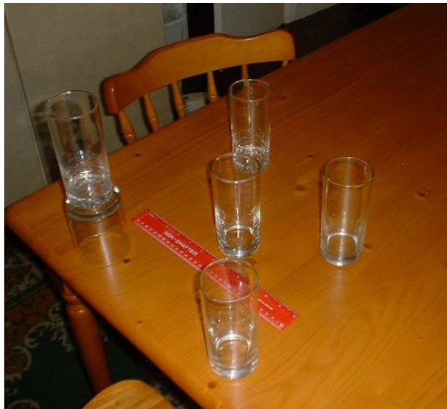
Plate 14 A home experiment to recreate the perspective distortion of an air photo.
