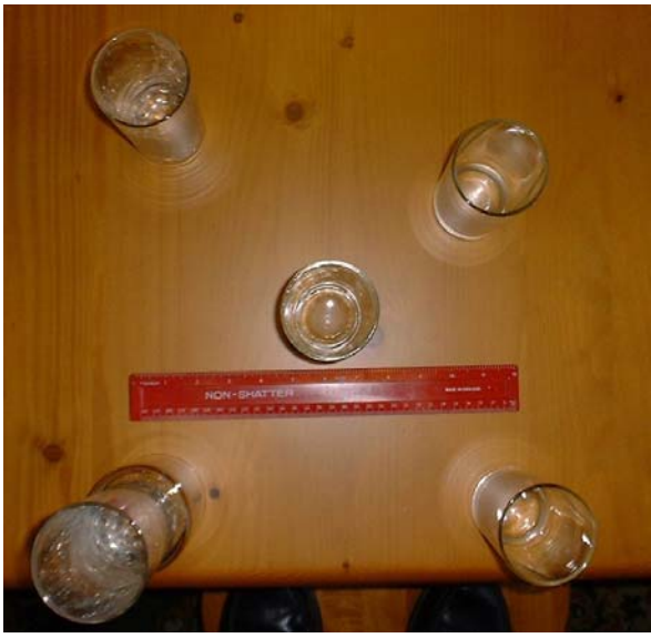
Plate 14 A home experiment to recreate the perspective distortion of an air photo.
