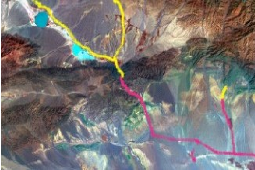
Plate 6 A query on GPS fixes from the Bogda Shan expedition: locations above 1,000 m are selected in a lighter colour (top half of the image); locations below 1,000 m are displayed but not selected (lower right of image).
