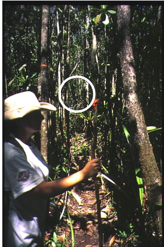
Plate 19 Compass traverse and slope inclinometer survey in dense jungle, Guyana. Note the problem of inter-visibility: photo (b) is looking back along the survey line towards the surveyor in the white T-shirt (circled) of photo (a).
