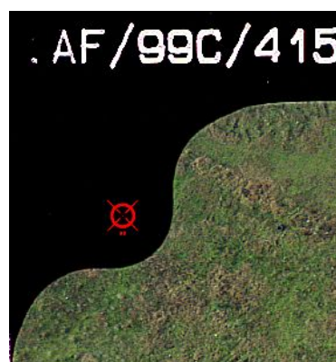
Figure 9-7 Example of a fiducial mark at the corner of an aerial photograph. There can be four or eight of these marks at the corners and in the centre of edges of photos, dependent on the camera make and model.
