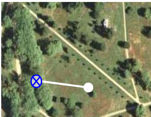
Plate 5 Using surveying techniques with a GPS to improve fixes in difficult locations. Top: a GPS reading is required at the blue cross under the tree cover. However, a few metres to the east the sky is not obscured by trees: the accuracy of the fix here will be an order of magnitude better. Lower diagrams: the receiver has been taken into the open and a reading taken. A compass has then been used to site the actual location required and a measurement has been taken along the line between the two points; this can then be plotted back into the GIS later.
