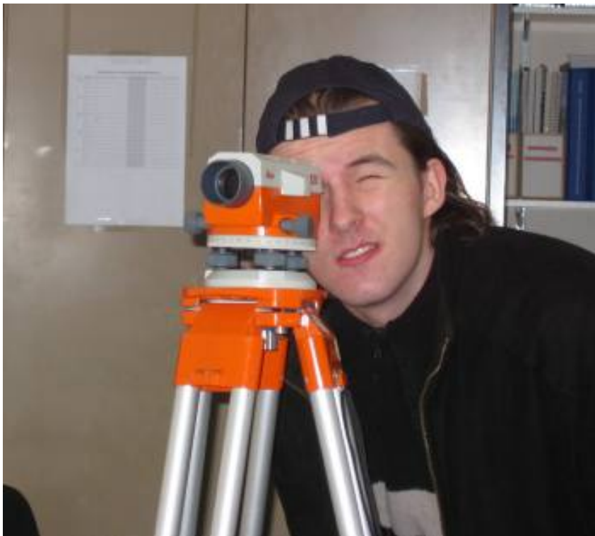
Figure 10-1 Sighting through a level mounted on a tripod.
