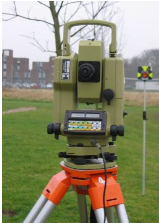
Figure 10-2 Total station mounted and ready to use on tripod. Note the use of a prism with this system. LCD display shows Easting and Northing of prism position.
