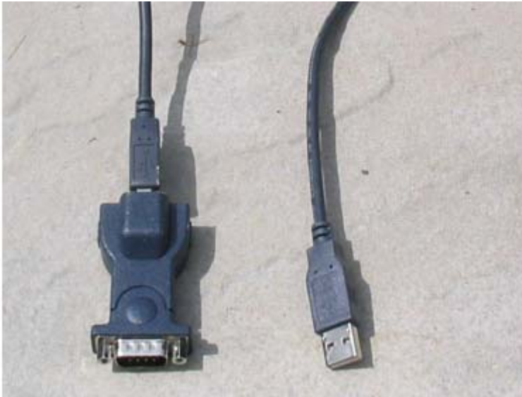
Figure 11-2 Serial - RS232 9 pin male to USB converter. The RS232 serial connector is shown on the left and the USB connector is shown on the right. The RS232 connector receives the female GPS connector and transfers the data through the USB port of the PC.
