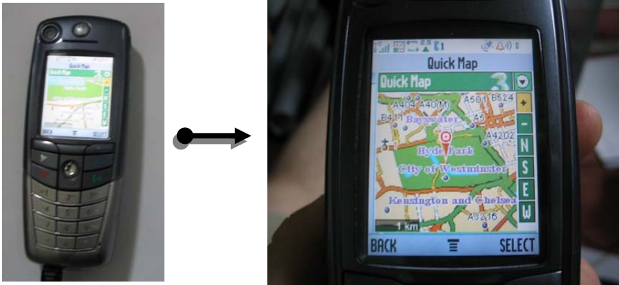
Figure 11-7 The use of Assisted GPS on a smart phone. This can give reasonable accuracy even in areas where normal GPS signals do not reach. However, it is expensive and poorly suited to most expeditions. A better solution for areas of poor signal strength is an external antenna connected to a standard receiver or a SIRF III 20 channel receiver.
