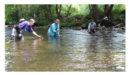
It may also be useful to measure velocity at different points across the river. Flow velocity may be faster or slower, depending on channel depth, inner or outer bend of a channel, vegetation growth and/or other obstacles.
