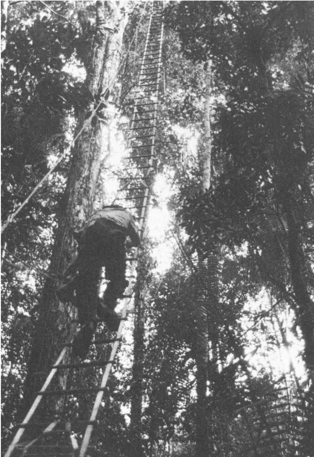
Figure 6.1 Tensioned webbing tape ladder for ascent to platform. Note safety line. Photo: A. Mitchell.
