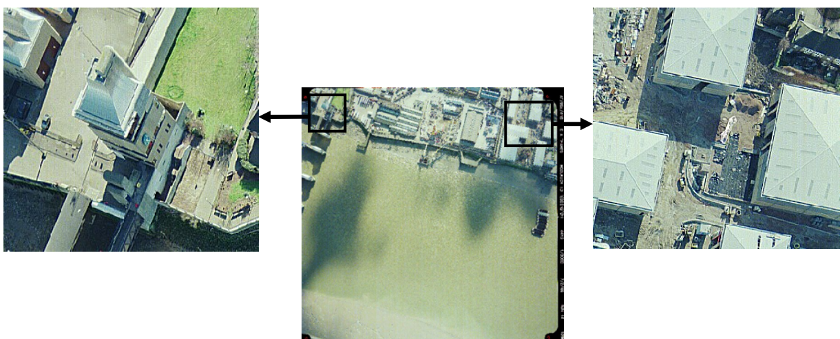
Figure 9-3 Radial distortion effects on buildings. Note how the buildings appear to lean away from the principal point (the photos are of the Thames Barrier, the river Thames and surrounding areas)
