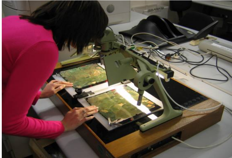
Figure 9-8 Air photo interpretation with a mirror stereoscope mounted on a light table (useful for viewing transparent air photos, diapositives, as well as traditional photographic prints).
