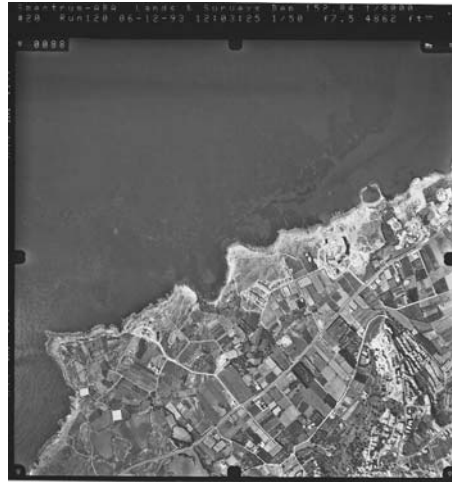
Figure 9-5 Example of a Black and White (panchromatic) aerial photo with title strip information.
