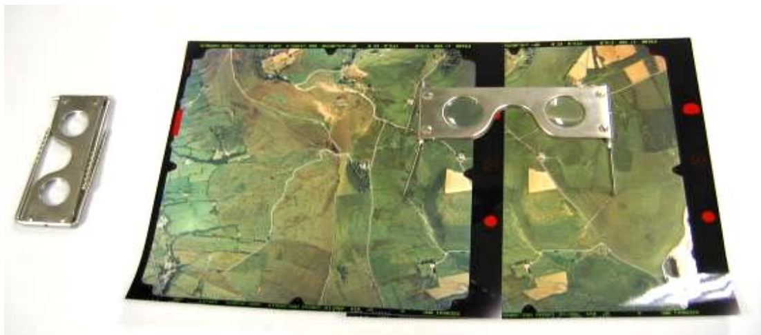
Figure 9-9 Pocket stereoscopes and aerial photo stereo-pair, one stereoscope set up for use, the other folded for transport. Photos are 9" per side for scale.
